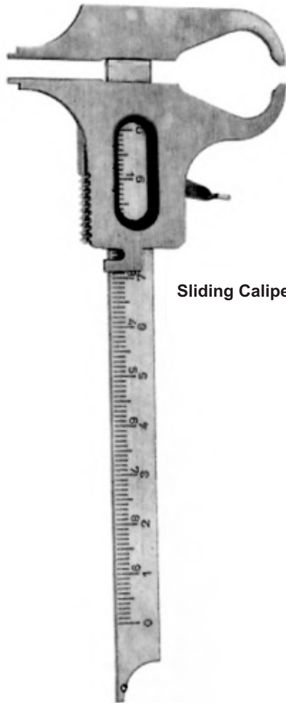
Boley NST/294 Measuring range } 0 - 100mm
